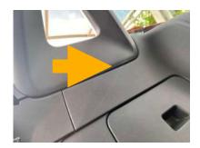
●At first look at the seatback bezel from below. There is one slit to insert the interior removal.
