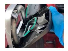
When the bezel comes off, the bezel blocker acrylic is at the rear of the vehicle body. (visible from behind), set the bezel blocker and replace the bezel to complete the work.
