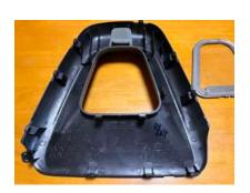
Finally, there are also claws around the bezel blocker, so the entire bezel is pressed down to make sure the claw points are tight together, and the work is complete. Thank you for your hard work in installing the seatback bezel!
